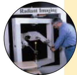
Source Imaging Goniometer manufactured by Radiant Imaging and used for creating Radiant Source Models
